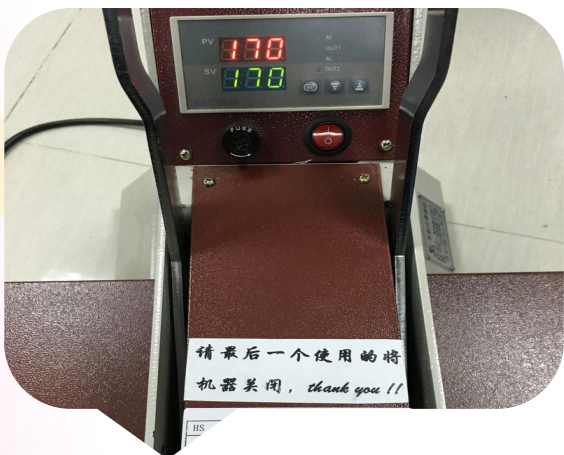
Preheat press machine suggested at 170°C(338F), 10 seconds
