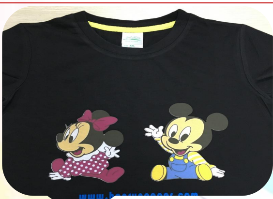
Preheat press machine suggested at 170°C(338F), 10 seconds
