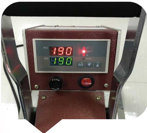
Preheat press machine suggested at 190°C(374F), 15 seconds
